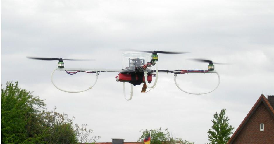
**Figure 1.** The Ifigicopter equipped with humidity and temperature sensors.
